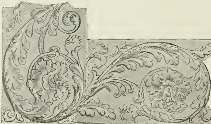
No. 116.—INTERNAL MITRE OF SOFFIT ENRICHMENT.
